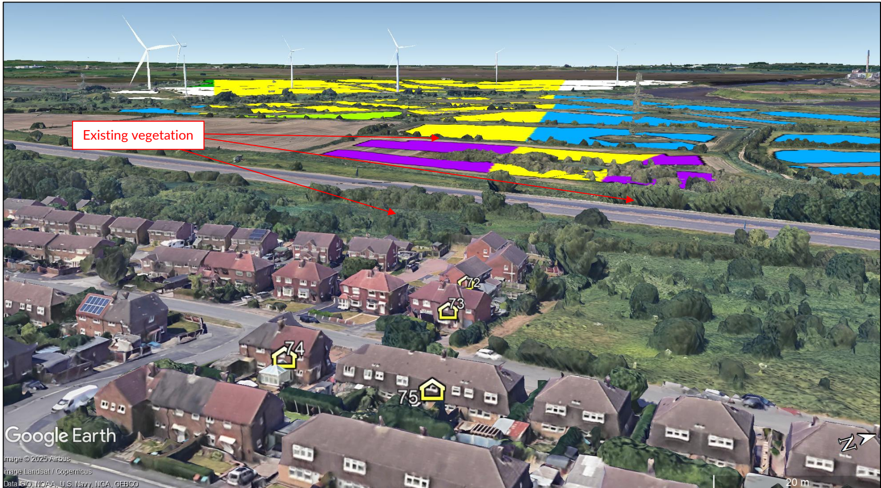
Figure J79 Reflecting panel area and partial screening for dwelling receptors 72 to 75
