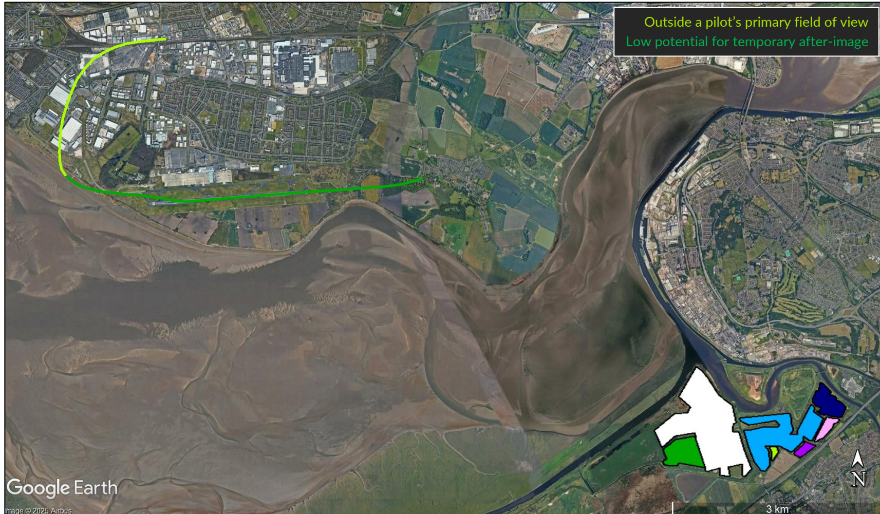
Figure 24 Solar reflections towards 09LH/ 27RH visual circuit
