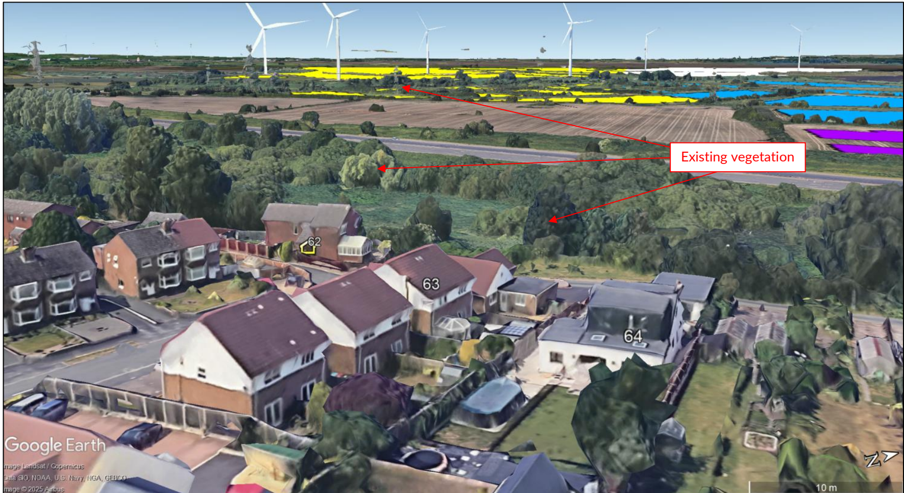
Figure J77 Reflecting panel area and partial screening for dwelling receptor 62 to 64
